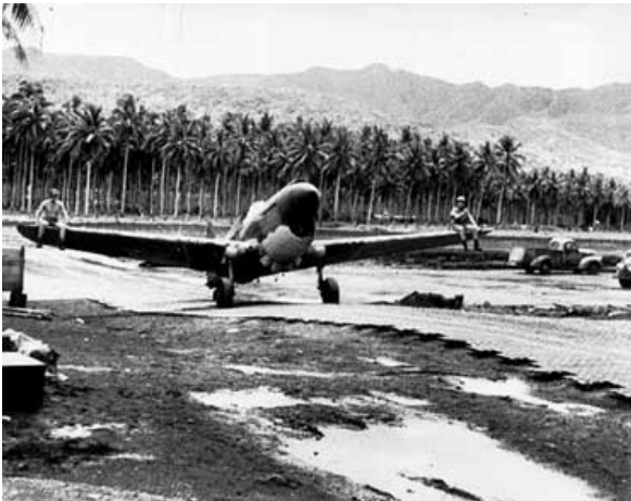
The airstrip at Milne Bay, left, as with all of the jungle strips in New Guinea was constructed of interlocking mesh. In the rainy season it tended to sink into the mud.
